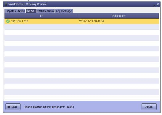
**Step 7** Click the "Dispatch Station" tab to check the connection status of the repeater.
