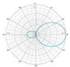
If the antennas are mounted for vertical polarization, these curves show the radiation patterns in the vertical
