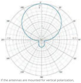
If the antennas are mounted for vertical polarization, these curves show the radiation patterns in the horizontal plane (horizontal coverage).
