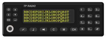
\*Menus that are accessible from the keypad: DTMF, Abbreviated Number List, Data Telegram, TX Power, Programming, Setup & Service.
