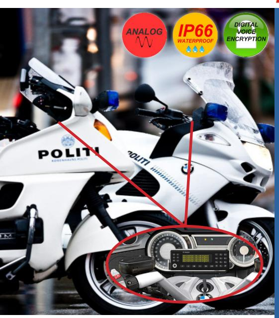
The TP6000i for motorcycles is a standard TP6000i mobile tranceiver with the waterproof BE905 Control unit. The control unit can be mounted directly on the radio or by distance from the radio unit via an RS232 controller interface.
