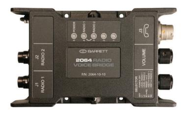
Cross-connecting the audio between network 1 and network 2 forms a bridge between the radio networks over which the 2064 user can both monitor and communicate. The voice bridge is automatically activated whenever voice is detected on either network.
