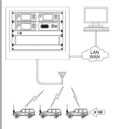
This scenario has 100 mobile transceivers, each with 3 channel programmed for GPS Push transmission. Each GPS Push transmission in this scenario takes approximately 10 seconds (assuming an antenna with memory tune is fitted).
