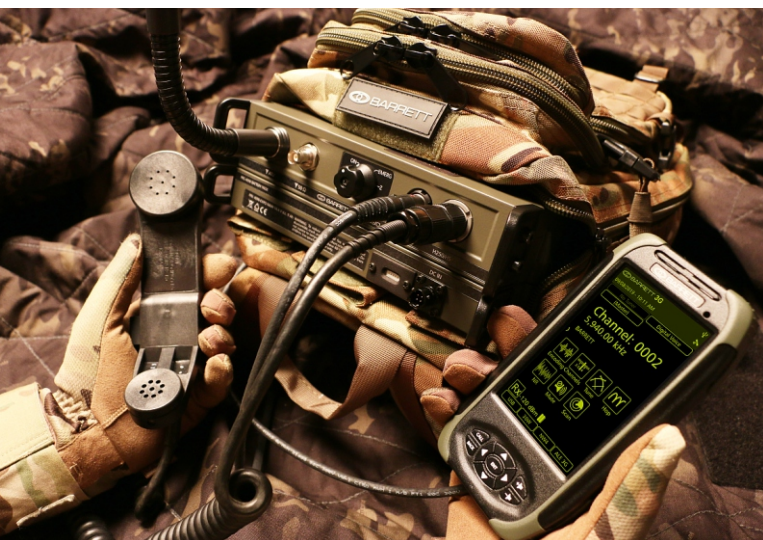
Barrett PRC-4090 HF SDR manpack with multicam daypack and optional H250 handset.
